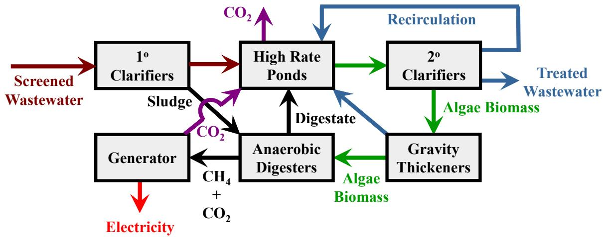
**Figure ES1:** Process schematic for Case 2 (wastewater treatment-emphasis with production of biogas only). The cases with a wastewater treatment-emphasis discharge large quantities of treated wastewater as the main facility product. ( $1^{\circ}$  = Primary;  $2^{\circ}$  = Secondary.)
