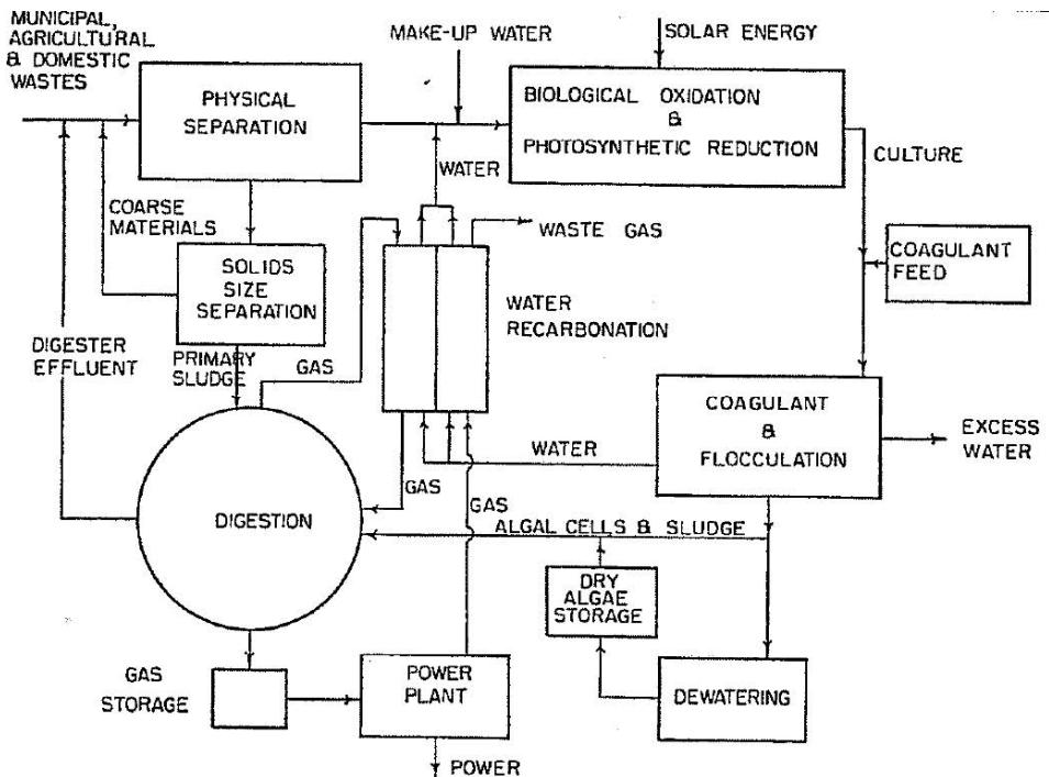
Figure 3.1: Algae-Methane–Electricity Process Schematic (Oswald and Golueke, 1960).
