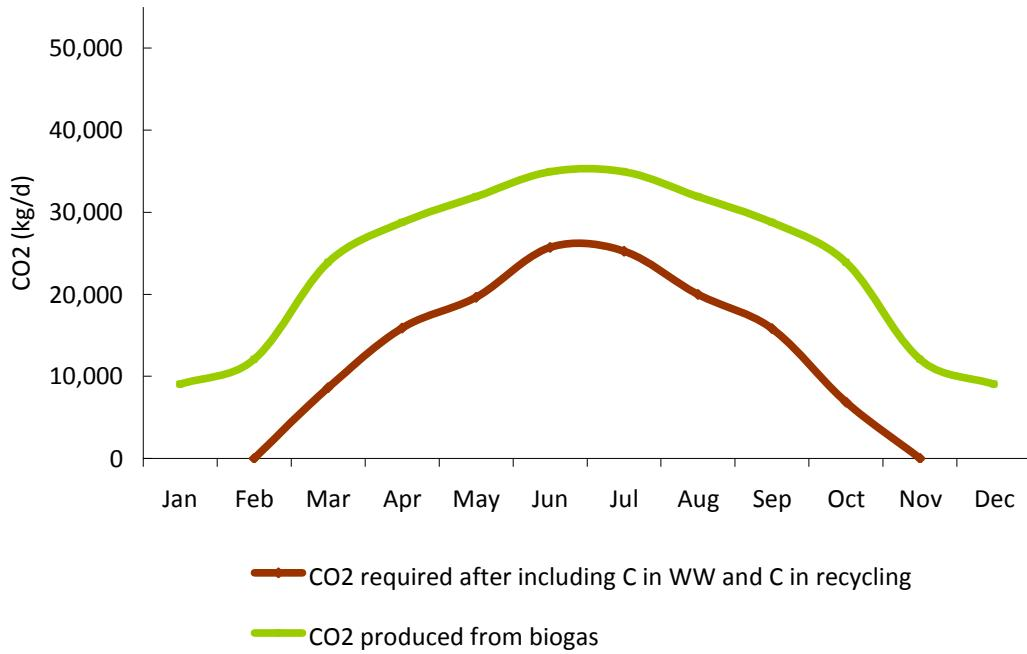
**Figure 5.18: Case 2 CO<sub>2</sub> Requirement and CO<sub>2</sub> produced onsite. Requirement is accounted for carbon in wastewater and recycling of carbon in digester effluent, 2° clarifier supernatant, and gravity thickener supernatant.**
