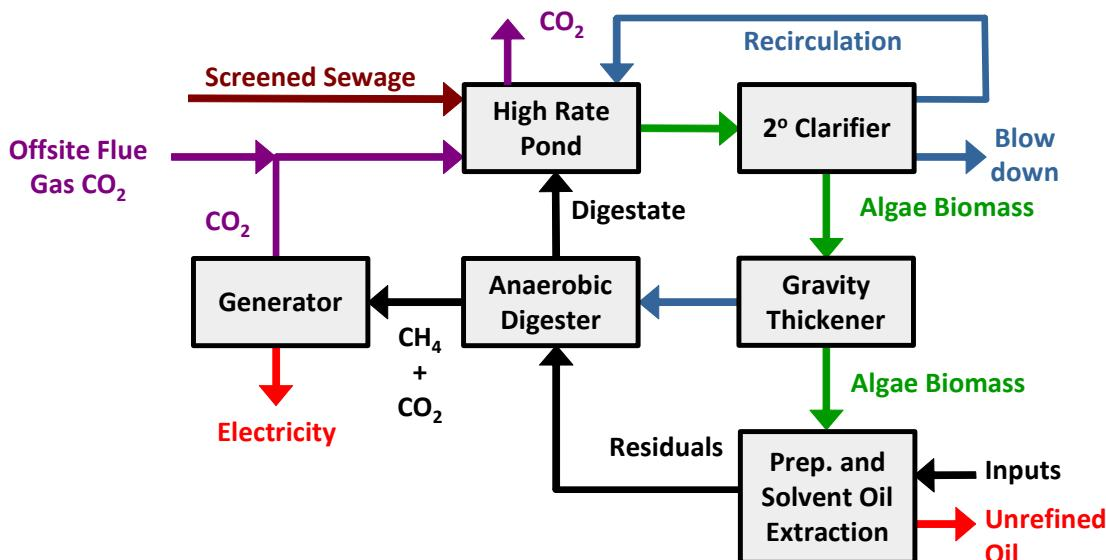
Figure 5.22: Process schematic for Case 3 (biofuel-emphasis + oil)
