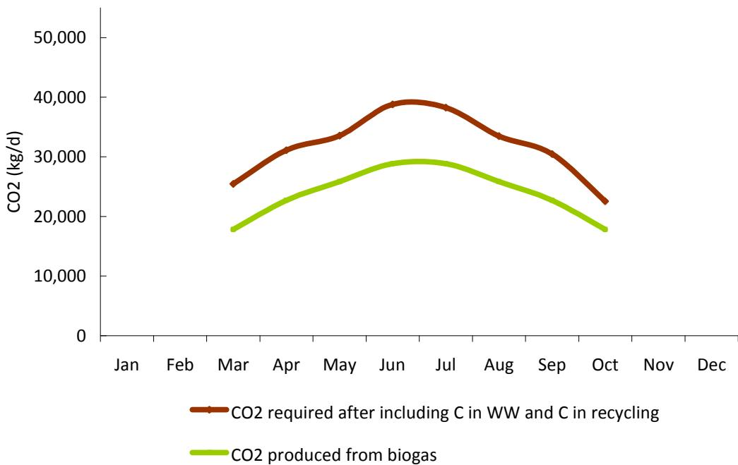
**Figure 5.25: Case 4 CO<sub>2</sub> requirement and CO<sub>2</sub> produced onsite. Requirement accounted for carbon in wastewater and recycling of carbon in digester effluent, 2° clarifier supernatant, and gravity thickener supernatant.**
