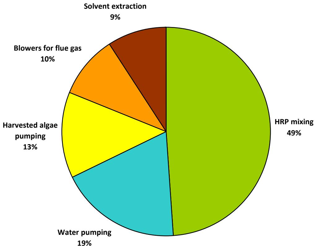
**Figure 5.16: Parasitic energy requirements breakdown by operation for Case 1 (100-ha)**
