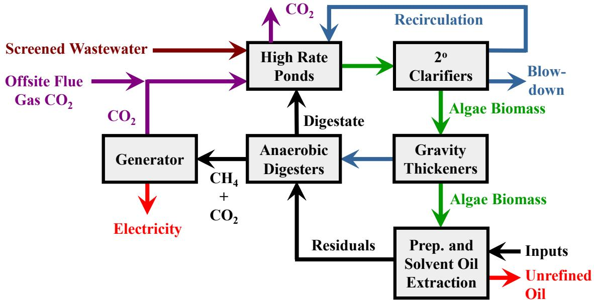
**Figure ES2:** Process schematic for Cases 3 and 5 (biofuel-emphasis with both oil and biogas produced). The cases with a biofuel-emphasis discharge a relatively small amount of water as blowdown, with most of the microalgae growth medium being recycled. A shared, centralized biomass preparation (cell disruption) and solvent extraction plant is included.
