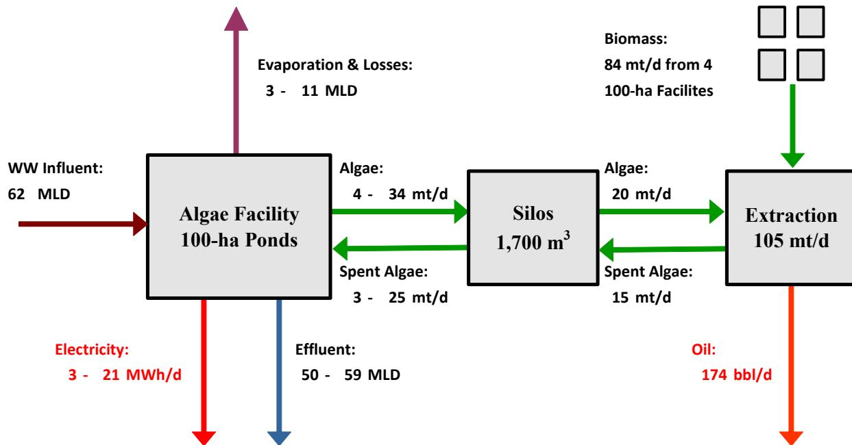
**Figure 5.19: Simplified mass balance for Case 1 (Wastewater treatment-emphasis + oil), showing seasonal variations and fuel and electricity production.**
