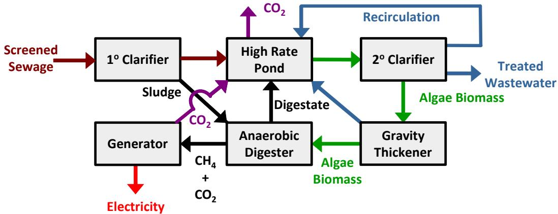
**Figure 5.14: Case 2 Process Schematic (wastewater treatment-and biogas production).**
