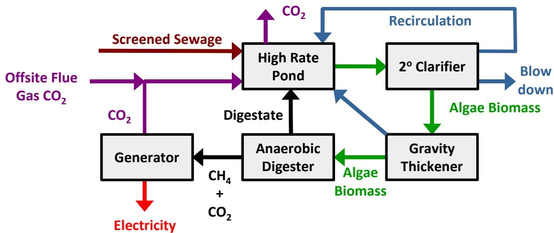
**Figure 5.23: Process schematic for Case 4 (biofuel-emphasis + biogas)**
