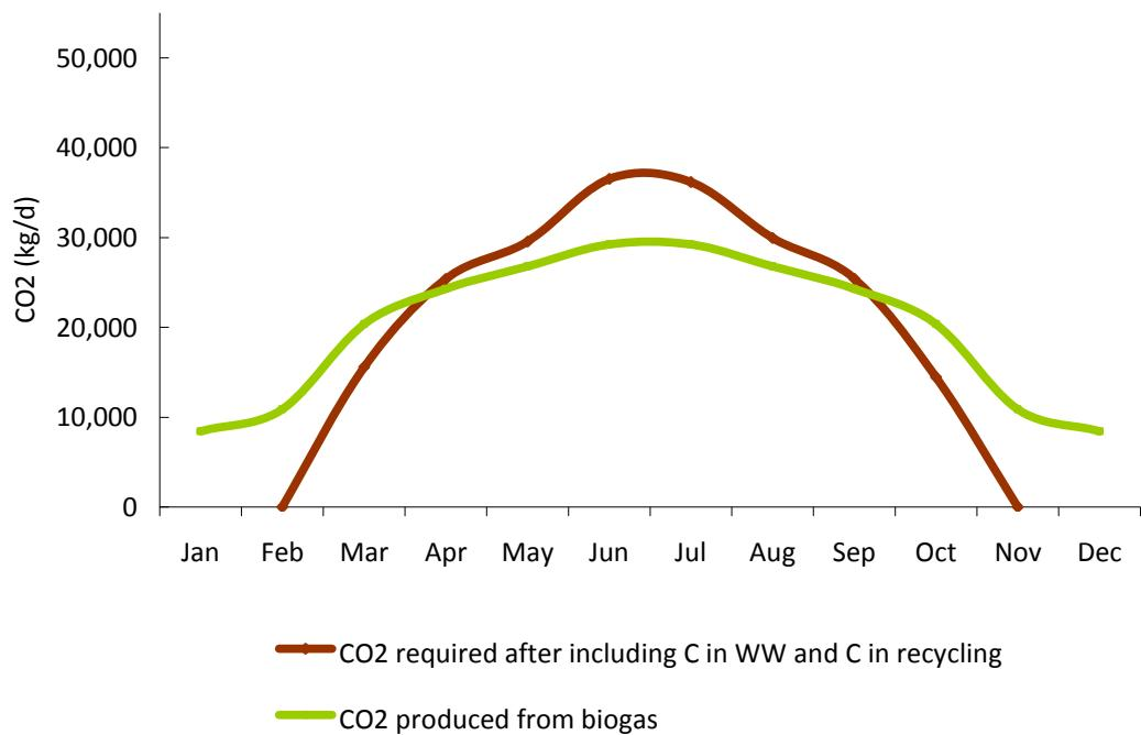
**Figure 5.17: Case 1 CO<sub>2</sub> Requirement and CO<sub>2</sub> produced onsite. Requirement is accounted for carbon in wastewater and in the recycling digester effluent and 2° clarifier supernatant.**
