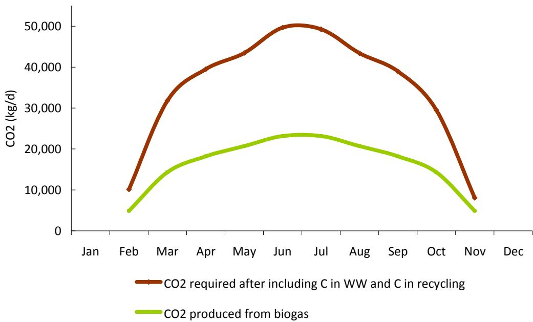
**Figure 5.24: Case 3 CO<sub>2</sub> requirement and CO<sub>2</sub> produced onsite. The requirement accounted for carbon in wastewater and recycling of carbon from digester effluent and 2° clarifier supernatant.**
