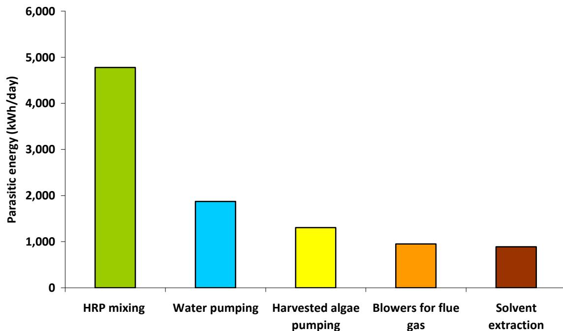
**Figure 5.15: Parasitic energy requirements for Case 1 (100-ha)**
